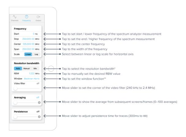
Note that [Start, Stop] and [Center, Span] in the frequency panel are equivalent representations of the measured frequency range. Moku:Lab will automatically update the other pair if one is changed.
