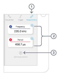
The measurements menu allows you to measure up to seven attributes at a time across both input channels and the math channel.
